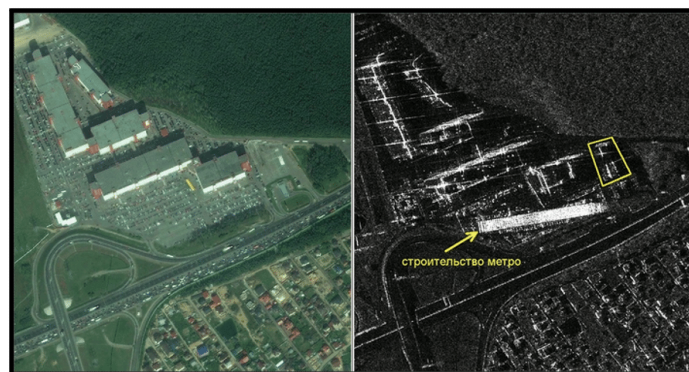
Figure 4: Left: GeoEye optical picture. © 2011 DigitalGlobe Inc., @ 1m res. Official distribution- ScanEx RDC. Right: Radar picture from COSMO-SkyMed. © ASI, 2014. New buildings that had not yet been built in 2011 are outlined in yellow. Source: Geo for All, 'COSMO-SkyMed inizia a diffondere immagini radar attraverso ScanEX in Russia', 3 February 2014, www.geoforall.it/k4c3p .
